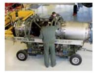
incorporates advanced technologies such as integrallybladed compressor disks, called 'blisks', low-pollution combustor, single-crystal high-pressure turbine blades, ceramic coatings, revolutionary powder metallurgy disks, and composite materials. Additionally, the M88 has been optimised so that its small infrared signature does not compromise the Rafale's overall IR signature, and its non-polluting, smoke-free emissions make the aircraft more difficult to detect visually than older designs.
