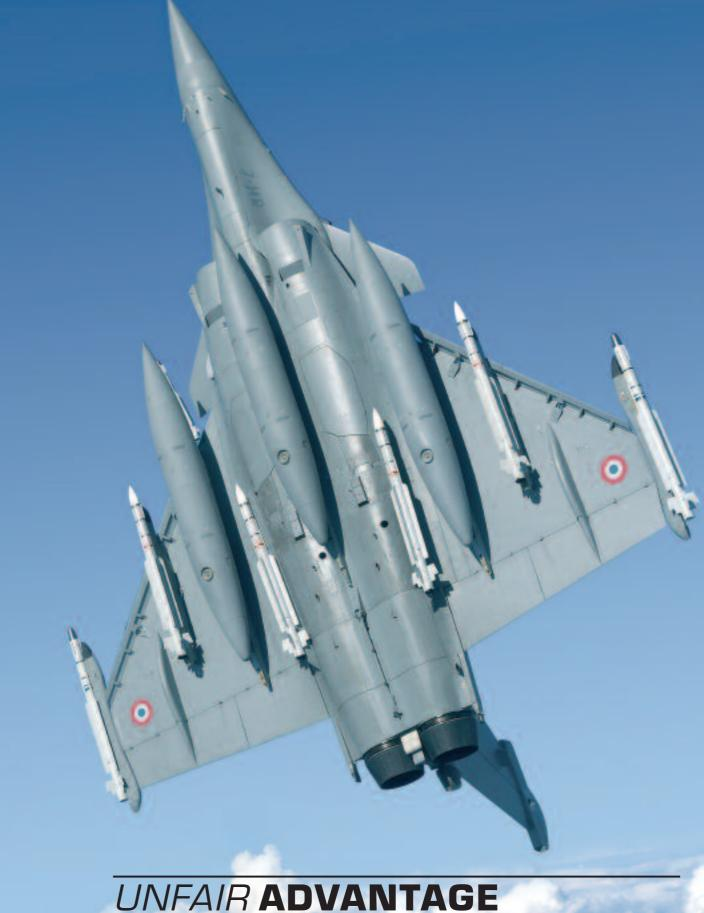
The Rafale omnirole fighter's main air-to-air weapon, the MICA (Missile d'Interception, de Combat et d'Autodéfense, Interception, Combat and Self-Defence Missile), is an advanced missile which provides unique capabilities. The fire-and-forget MICA was developed as a multi-target multi-mission multi-wave weapon to replace both the acclaimed short-range, IR-guided Magic 2 and the long-range, radar-guided Super 530D arming the Mirage 2000.
